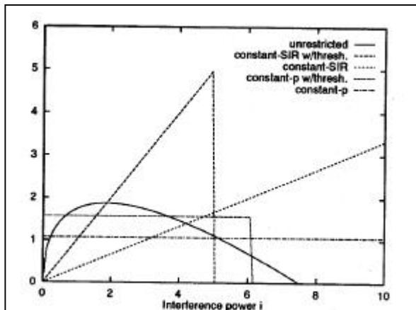
Figure 1: Transmitter power using various forms of power management. ((1), fig. 4)
