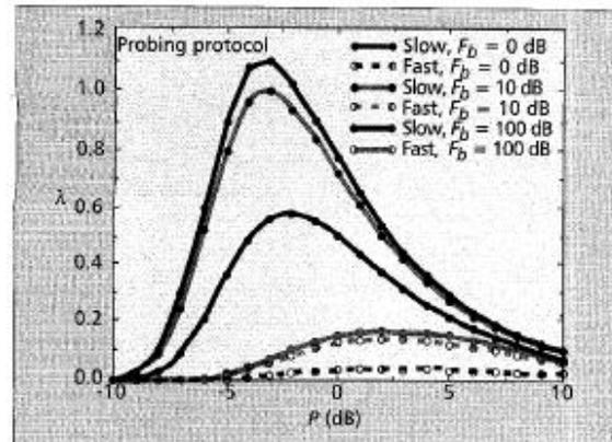
Figure 5: Energy efficiency vs. normalized output power for probing protocol with slow ( $f_b T = 0.02$ ) and fast ( $f_b T = 1$ ) Rayleigh fading. ((2), fig. 2)
