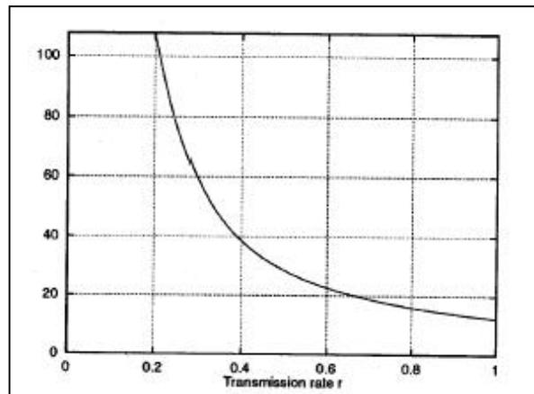
Figure 2: Percent increase in useful battery life using unrestricted power management versus best-case constant-SIR operation. ((1), fig. 3)
