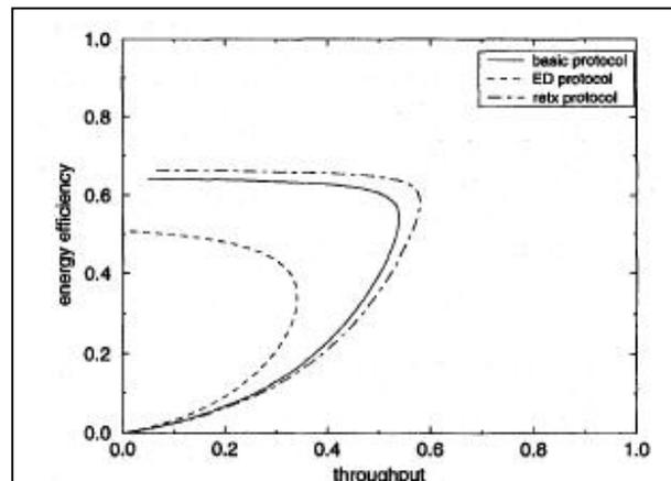
Figure 7: Energy efficiency vs. throughput for various protocols in fast fading, i.e.,  $f_b T = 0.64$ ,  $N = 10$ . ((3), fig. 2)
