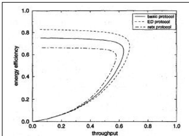
Figure 6: Energy efficiency vs. throughput for various protocols in slow fading, i.e.,  $f_b T = 0.02$ ,  $N = 10$ . ((3), fig. 1)
