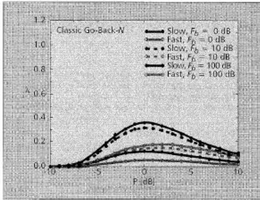
Figure 4: Energy efficiency vs. normalized output power for GBN protocol with slow ( $f_b T = 0.02$ ) and fast ( $f_b T = 1$ ) Rayleigh fading. ((2), fig. 1)
