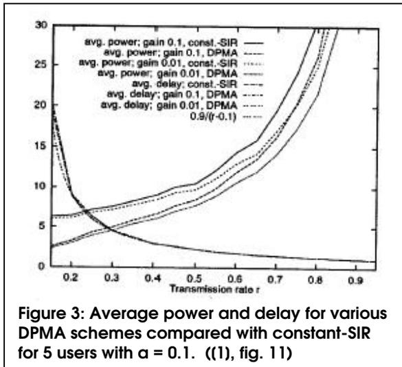
**Figure 3: Average power and delay for various DPMA schemes compared with constant-SIR for 5 users with  $\alpha = 0.1$ . ((1), fig. 11)**
